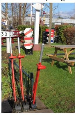
The two ground signals mentioned in 'Progress at the Box'. On the left is the repositioned triple 'dolly' now on the lawn and linked up to the recently installed third L&NWR lever. To the right is the BR Eastern Region/LNER signal that was originally Chesterton Junction north of Cambridge. This now works off the green lever of the MR ground frame.
