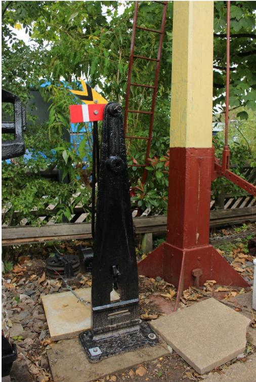
**Two recent additions to the garden display. On the left is the set of fog repeater signals originally located at Market Harborough. Replacement arms have been made and the equipment is linked to the adjoining home and distant signals. To the right is a milepost that stood at Coughton in Warwickshire on the line from Barnt Green to Ashchurch via Reddich. The distance was measured from a zero point at London Road Junction, Derby not St Pancras. Both items have been kindly donated to the Trust.**
