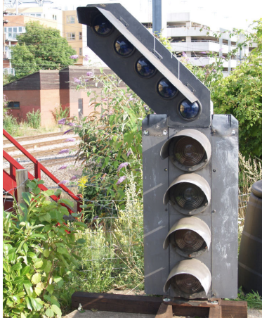
The 'feathers' or direction indicators now sitting on top of one of the four aspect signals in the garden
