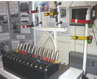
The miniature lever frame and signals in the locking room. 6 of the levers operate the signals and demonstrate the principals of interlocking to visitors.
